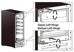
6. Loose the 2 screws with a cross screwdriver. Keep these screws and the handle well on one side for using later.
