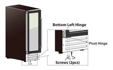
10. To reinstall the handle to the left top of door frame.
