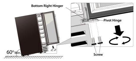
2. Carefully remove the door from the Upper Right Hinge and prevent it from scratching. Take out the Pivot Hinge from the door hinge hole.
